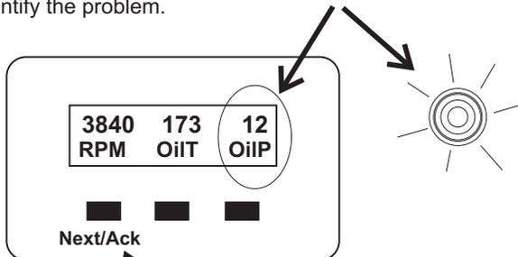
If the problem can not be solved, the pilot acknowledges the alarm with the Next/Ack (acknowledge) button. The warning light will stop flashing, but will remain illuminated until the problem goes away. The display page will return to the page it was previously on after the alarm is acknowledged.
