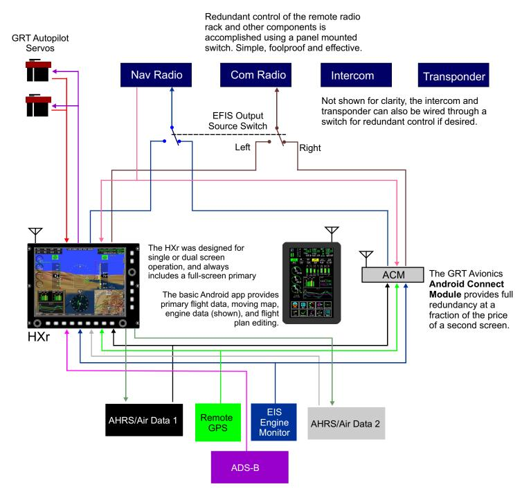
The HXr's 8 serial inputs/outputs allow a high degree of functionality and redundancy. In this example an Android tablet computer is used to add redundancy and provide touchscreen control. In normal operation, the Android communicates directly with the HXr for display and control. In the event the HXr was non-functional, the optional Android Connect Module (ACM) allows an independent means of interfacing the Android tablet to aircraft systems at a very attractive cost.
