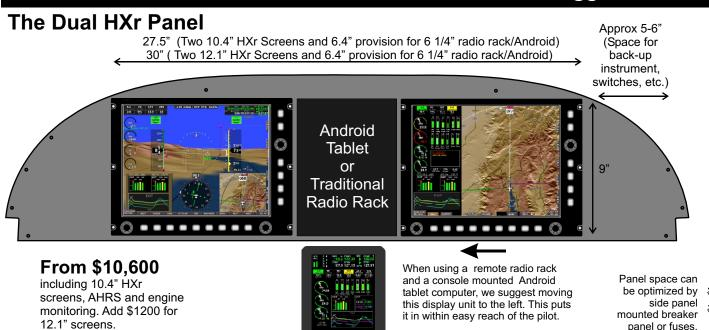
An RV-10 Panel easily accommodates two 10.4 or 12.1" HXr screens with room for a large Android Tablet or a traditional radio stack. (RV-6,7,9 can easily accommodate two 10.4" HXr screens.) If a traditional radio stack is used, an Android can be mounted in the console. Significant panel space remains for mechanical backup instruments and switches. Android table computer also allows control of remote radio rack.
