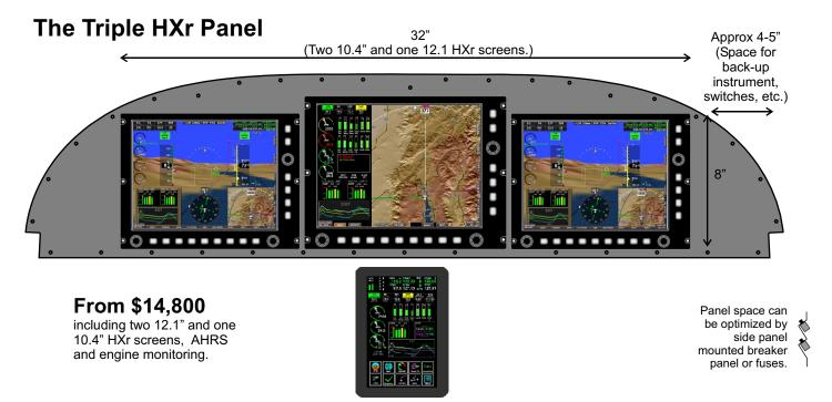
A spectacular 3-screen EFIS system at a surprisingly affordable price. Full remote radio rack, large (12."1) screen typically would serve as moving map/chart viewer, with 10.4" screens dedicated to each pilot. Console mounted android for touch panel input and auxiliary display. Significant panel space remains for desired backup instruments.
